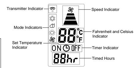
NOTE: If you used the control panel to set up the unit, the remote control will not automatically update the information shown on the remote control's LCD.
